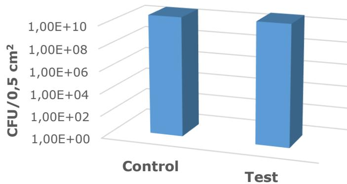
**Figure 1** Number of CFU in the drain pipe of both sinks before installing a UV bottom valve in the test sink and cleaning of control sink (0.5 cm<sup>2</sup>, depth: 6 cm).
